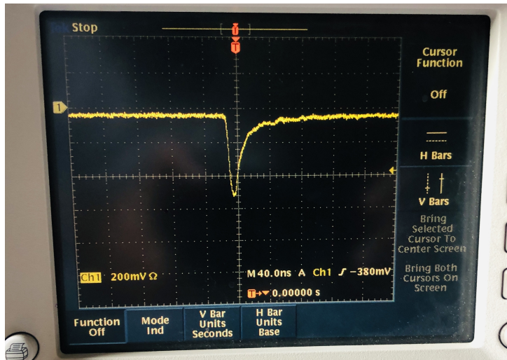
Figure 4.6. | Oscillogram of the scintillator signal of Top(A) PMT . The input impedance of the oscilloscope is 50\Omega , voltage scale is 200 mV/square, and the time scale is 40 ns/square. The trigger of the oscilloscope is set to -380 mV.
