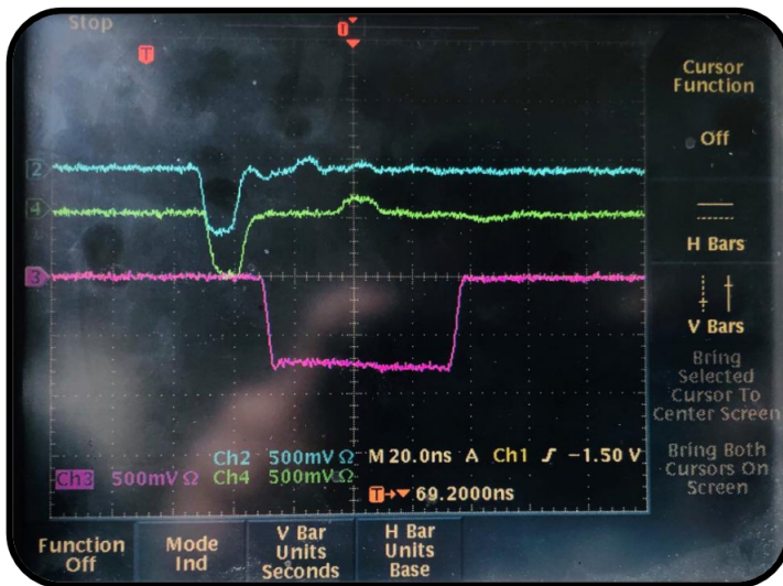
Figure 4.10. | Coincidence window (pink) of 70 ns with two digitized signal from PMT.
