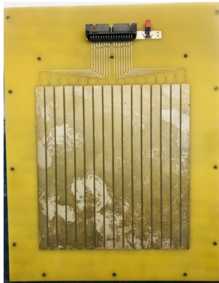
Figure 6.1. | Readout board (V1.0) from with a degraded copper strips.
