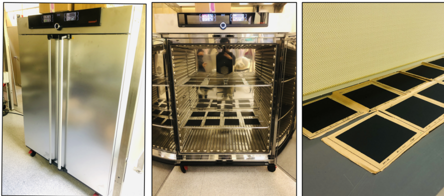
Figure 5.11. | UF750plus lab oven (left). Painted glass plates placed in the oven for curing (middle). The cured plates stored in a white room after measuring the resistivity (right).
