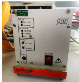
Figure 8.6. | fuG HCE 35-20000 high voltage power supply [123], this can reach high voltage of 20 kV from 0 V.
