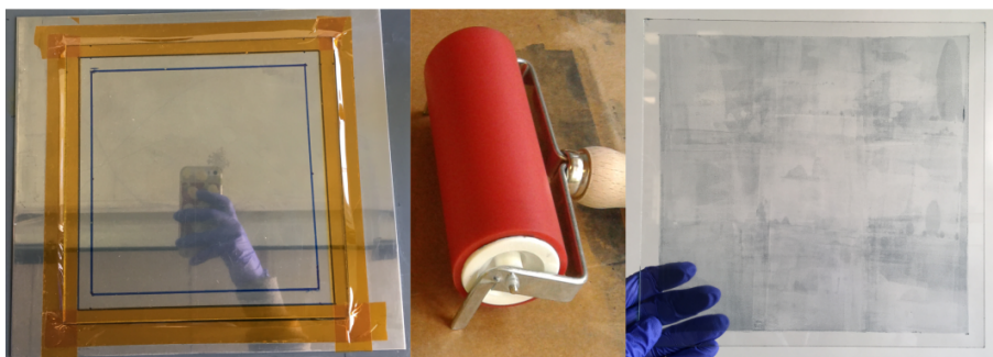
Figure 3.3. | Method to apply the resistive coating on glass plates, (left) Masked glass plate before applying paint, (middle) Roller used to spread paint, (right) Painted a glass plate. Figure from [99].
