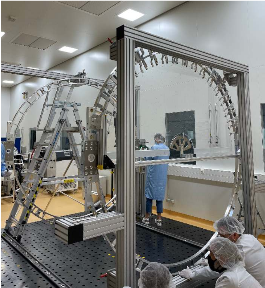
Figure 5.44. | A picture of the disk and double-disk assembly platform. The picture is taken during a workshop organized between the TEDD project collaborators hosted by DESY.
