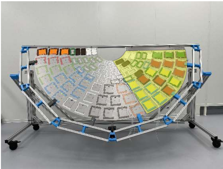
Figure 5.26. | The dee mockup on the dee integration table (the table in the picture is a temporary solution which will be replaced by the final design shown in Figure 5.2).
