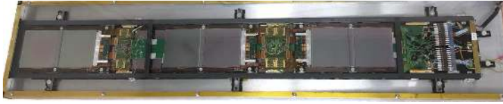
Figure 3.6. | The picture of an assembled TOB rod [20].
