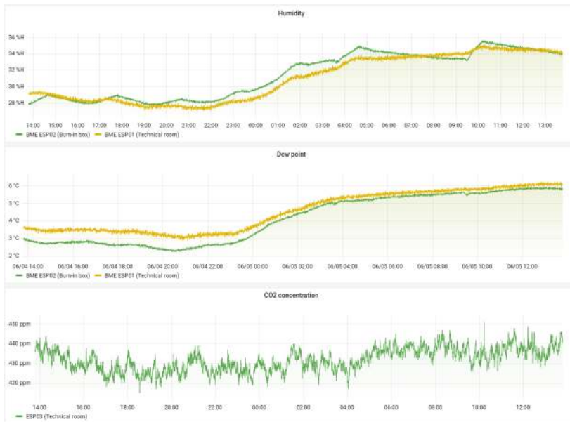
Figure 5.7. | The dashboard created with sensor readout: the humidity levels (top plot) and the dewpoint (middle plot) in the burn-in box and in the technical room, and CO 2 levels in the technical room (bottom plot).
