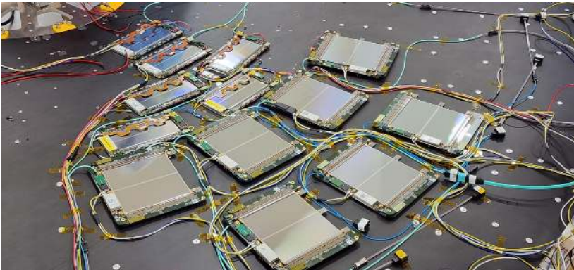
Figure 5.47. | Picture of a partly installed TEDD1 odd top Dee from the pre-integration test at DESY.
