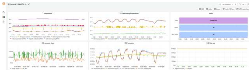
Figure 5.4. | The dashboards for MARTA parameters: temperatures, CO 2 pressures and flow rate, as well as the status summary is plotted.
