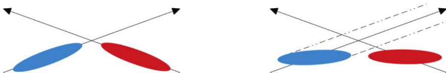
Figure 4.2. | Sketch of bunches colliding in a regular accelerator on the left, and with the introduction of crab-cavities to the right. From [51].
