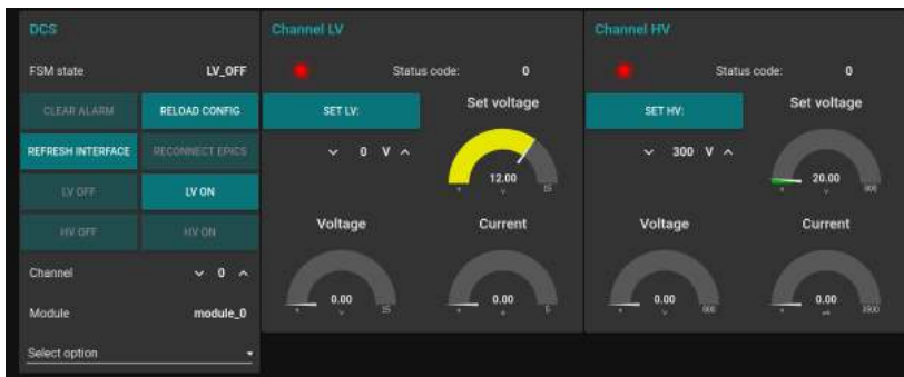
Figure 5.3. | The user interface for CAEN power supply. The DCS details with the FSM state is indicated on the left. The control of the LV and HV channels is indicated in the middle and on the right, respectively.
