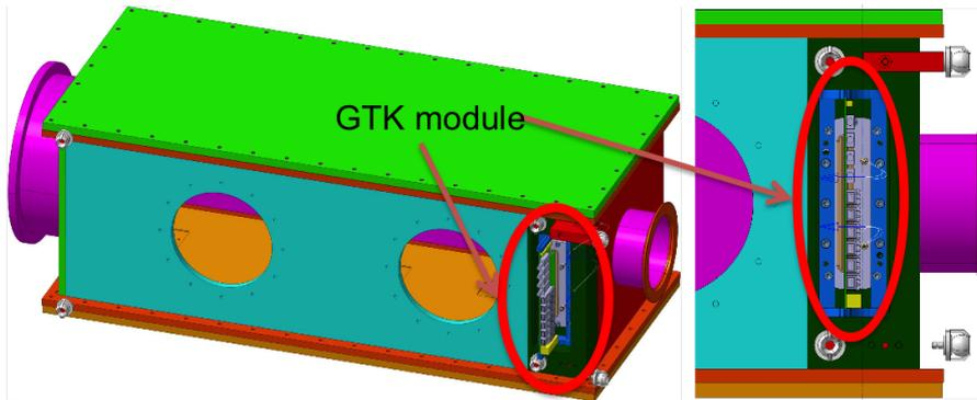
Figure 5.3: GTK module at position 3 integrated into the CHANTI vessel.
