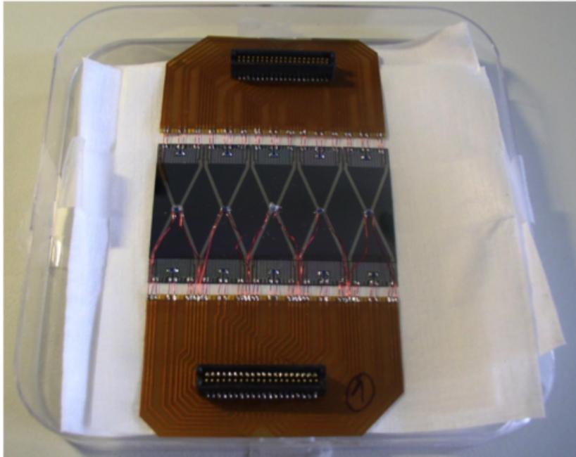
Figure 3.22: Silicon mock-up assembled and equipped with temperature sensors.
