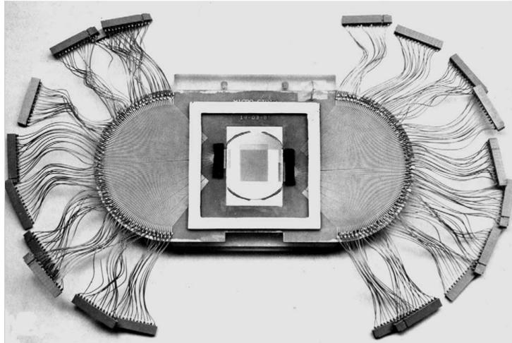
Figure 2.1: A mounted NA11 silicon strip detector [81].
