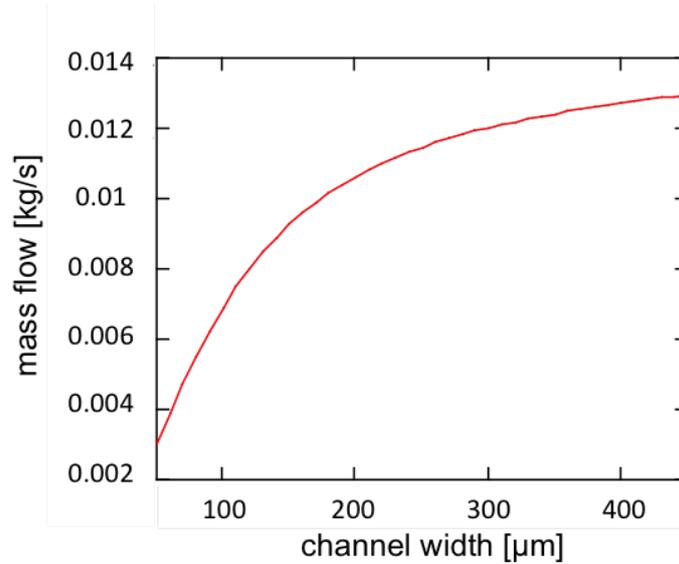
Figure 2.10: Mass flow rate of  $\text{C}_6\text{F}_{14}$  over channel width  $w$  for the GTK micro channel heat sink ( $h = 90\ \mu\text{m}$ ,  $\Delta p = 2\ \text{bar}$ ,  $b = 3/2 w$ )
