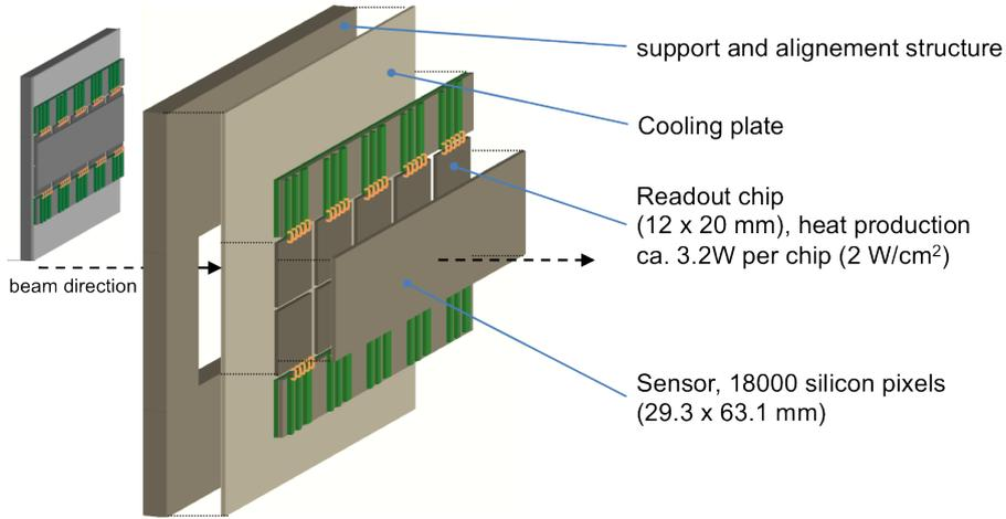
Figure 1.5: Schematic view of one GTK module
