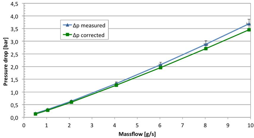
Figure 4.14: Measured pressure drop of the alternative cooling frame at  $-20^{\circ}\text{C}$  fluid inlet temperature. The error bars on the measured values are magnified 10 times to make them visible.
