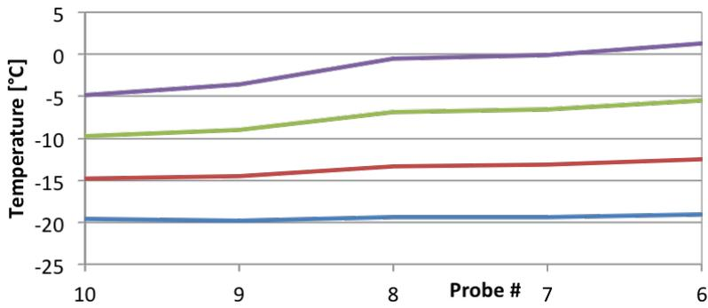
Figure 4.17: Temperatures of the analogue part for different power settings.
