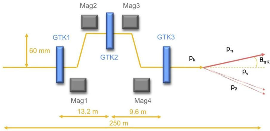
Figure 1.4: Layout of the GTK stations
