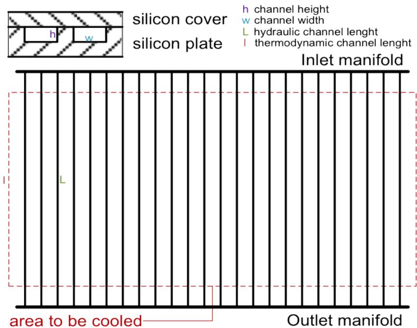
Figure 2.9: Micro channel layout with the important dimensions
