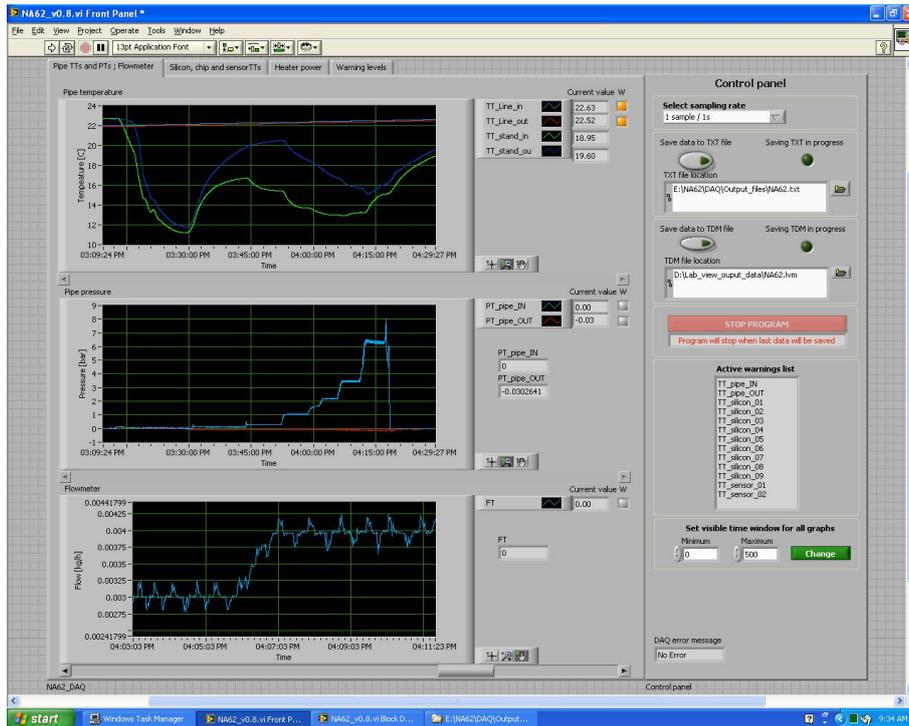
Figure 3.29: DAQ: LabView graphical user interface
