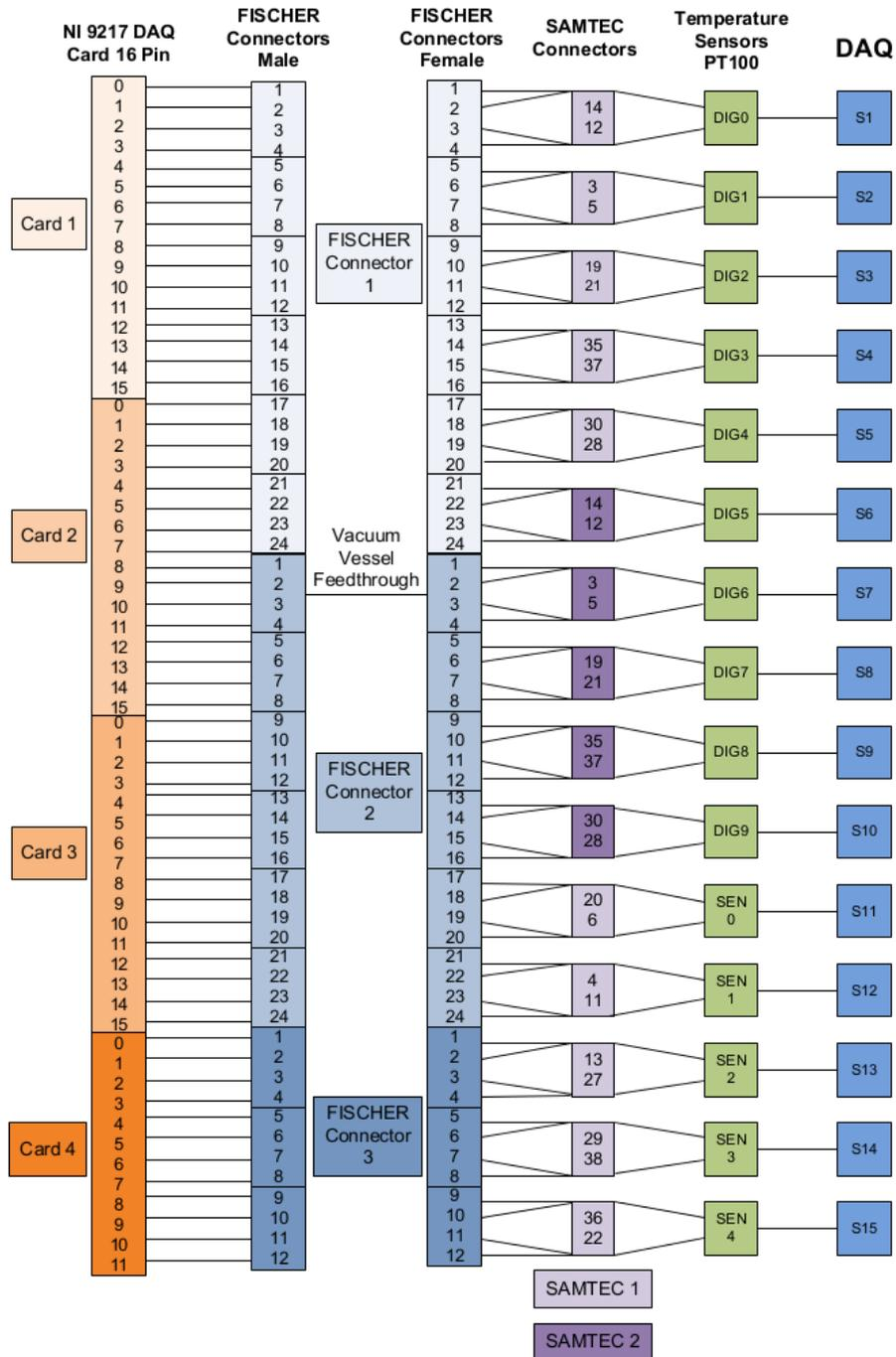
Figure 6.3: Wiring scheme for the electronics mock-up.
