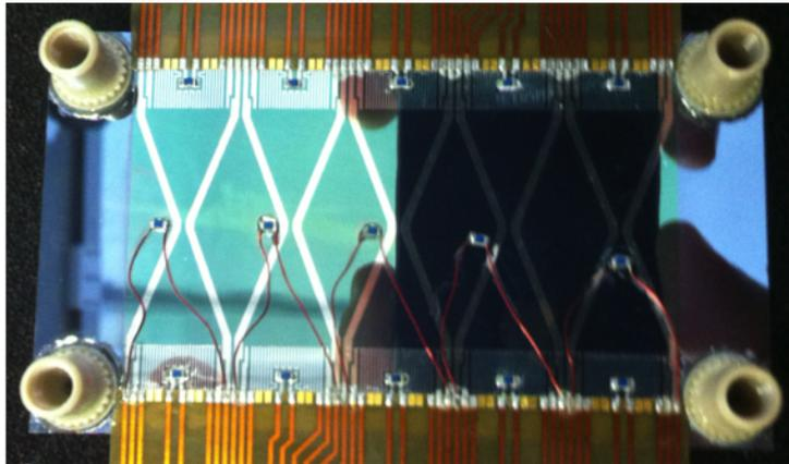
Figure 3.16: Micro channel frame with inlet/outlet connectors and silicon mock-up glued on top. The coolant runs horizontal from left to right or vice versa under the EoC region.
