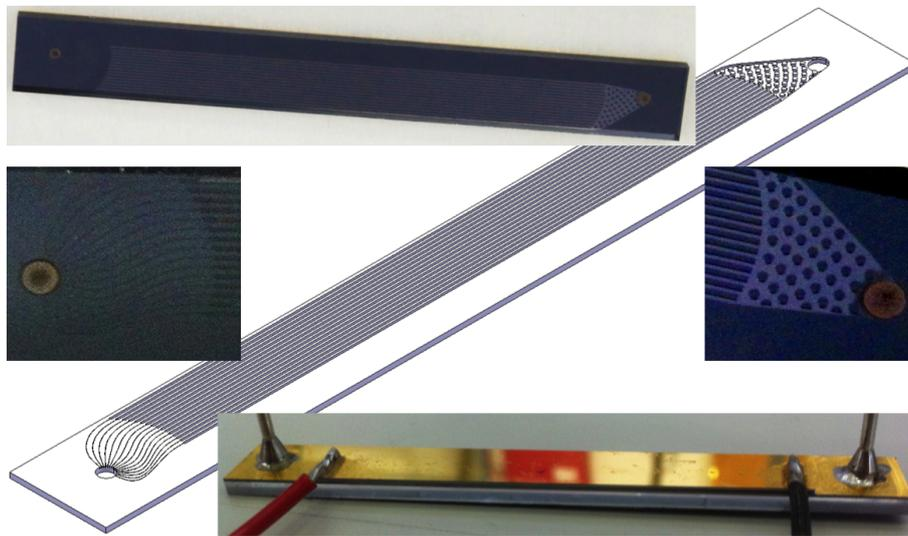
Figure 4.29: Cooling frame stave with micro channels for CO<sub>2</sub> and solder connectors, see 5.2.1.
