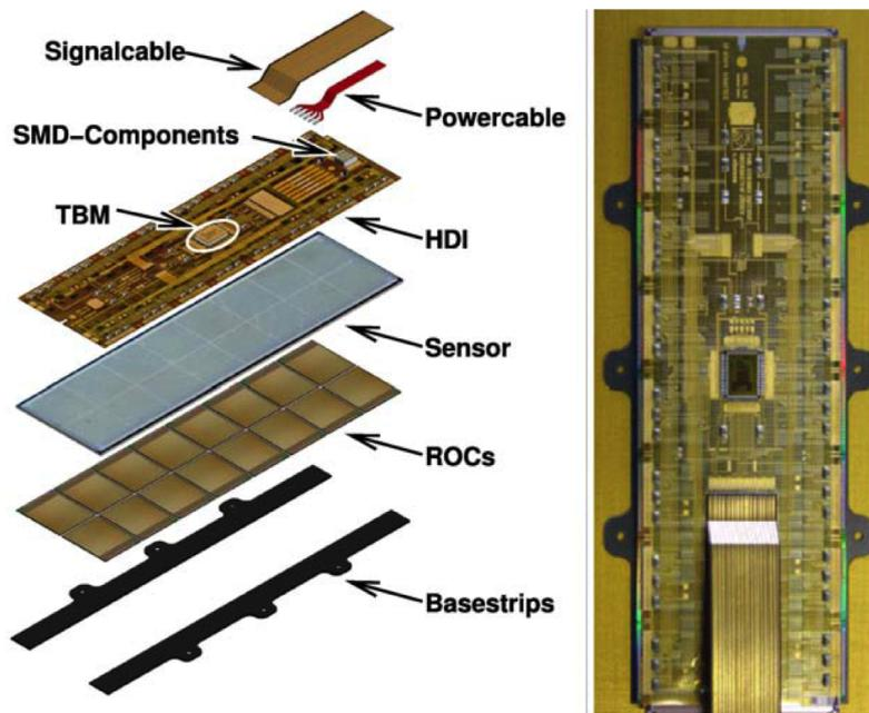
Figure 2.2: A CMS inner tracker pixel module [30].
