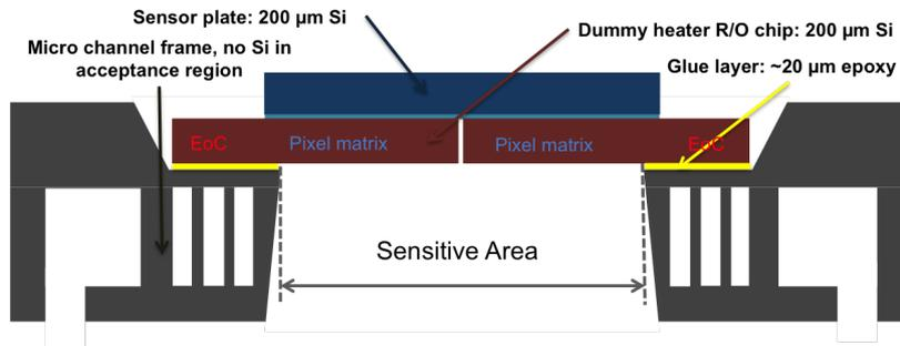
Figure 3.11: Schematic of the cooling frame with electronics.
