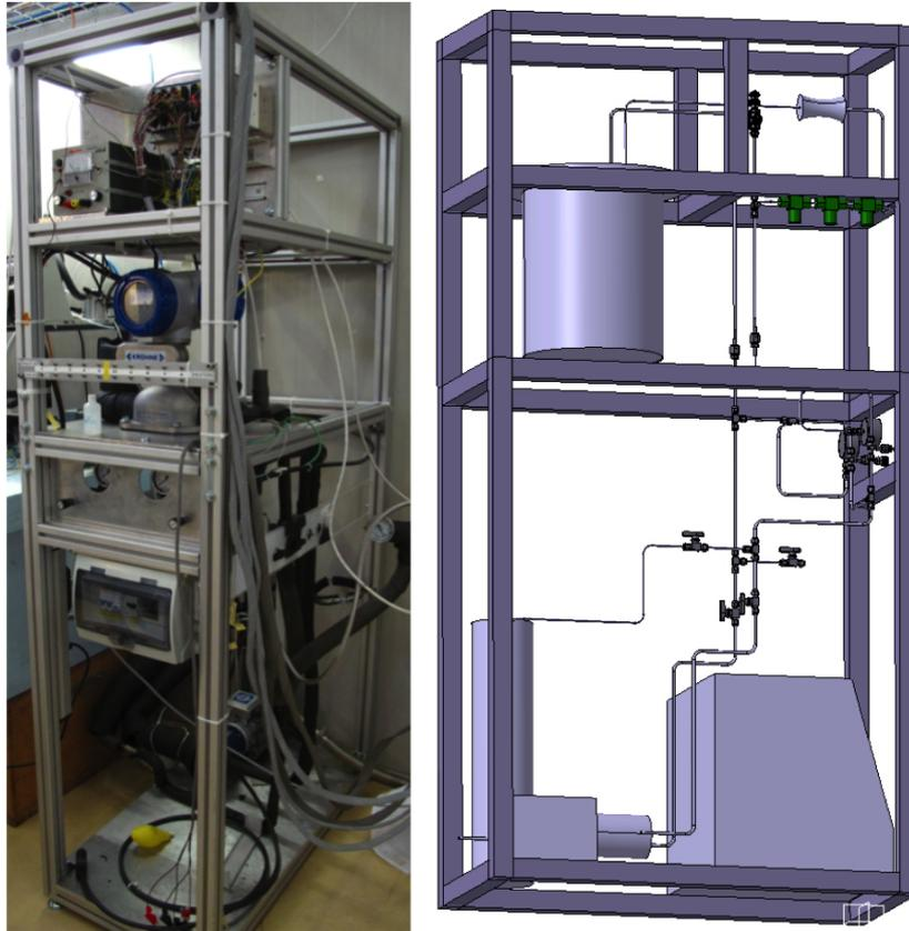
Figure 3.27: Micro channel cooling test rack in the lab and as 3D model
