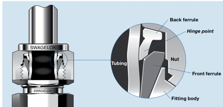
Figure 5.11: The principle of the Swagelok fitting connector [73].
