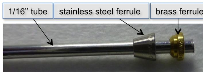
Figure 5.12: The Swagelok ferrules are used to create a solder-able surface.
