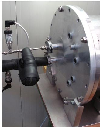
Figure 3.26: The lid of the vacuum vessel.
