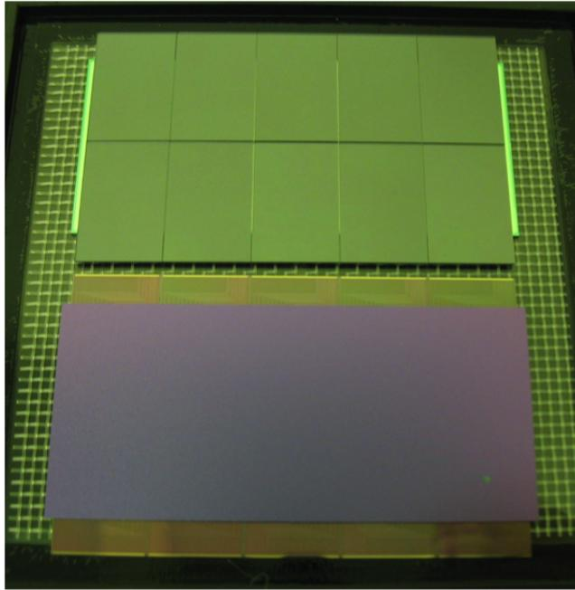
Figure 5.4: Sensor assembly dummy, used to verify the bump bonding process.
