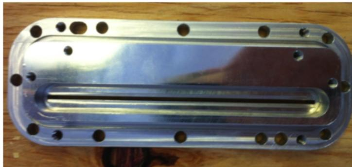
Figure 5.7: Flange for repeatable geometrical precision during installation.
