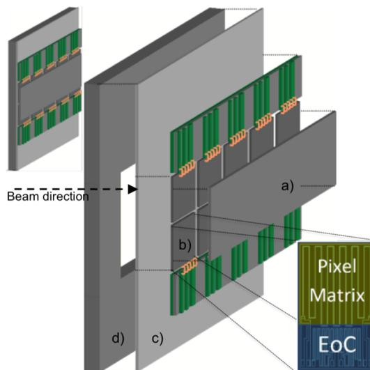
Figure 3.9: Schematic of the GTK subdetector and its readout chip TDC<sub>pix</sub>.
