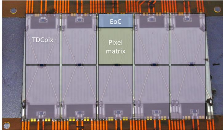
Figure 4.3: Mock-up electronics: configuration of the 10 TDCpix compared to the heaters on the mock-ups.
