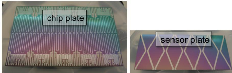
Figure 3.21: Silicon mock-up plates before glue assembly.
