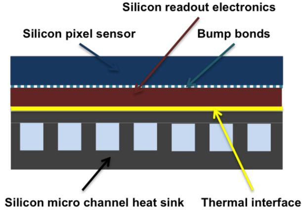
Figure 2.8: Principle of cooling with micro channels
