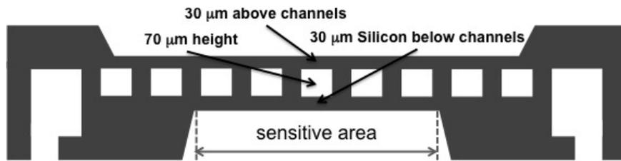
Figure 3.1: Schematic cross section of the baseline design
