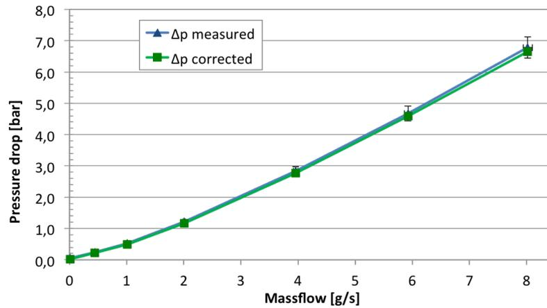
Figure 4.5: Measured and corrected pressure drop of the baseline cooling plate at  $-20^{\circ}\text{C}$  set point temperature of the cooling plant. The error bars on the measured values are magnified 10 times to make them visible.
