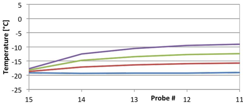
Figure 4.18: Temperatures of the lower digital part for different power settings.
