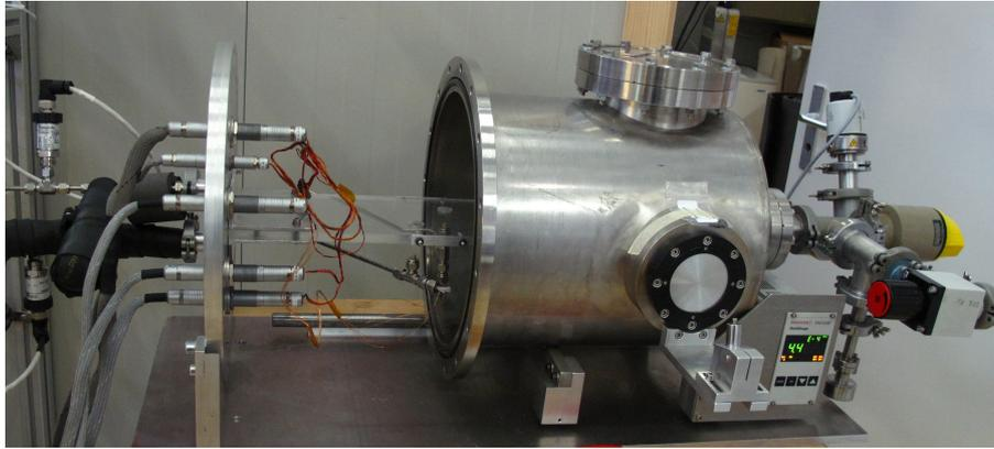
Figure 3.25: The vacuum vessel fully equipped before closing.
