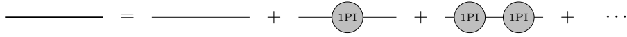
Figure 1.6: Geometric series of the Schwinger-Dyson equation (1.52). Thick (resp. thin) solid lines represent fully dressed (resp. free) propagators.
