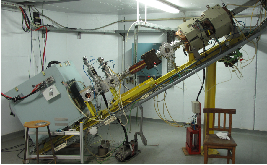
Figure 3.10: Photograph of the T2 beam line. The sample supports are slid between two copper plates inside the last vacuum chamber of the line. After the insertion, the chamber is closed and evacuated. The beam is going from the top right to the bottom left.
