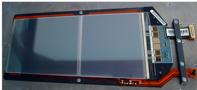
Figure 2.5: A TEC module and its reading electronics.
