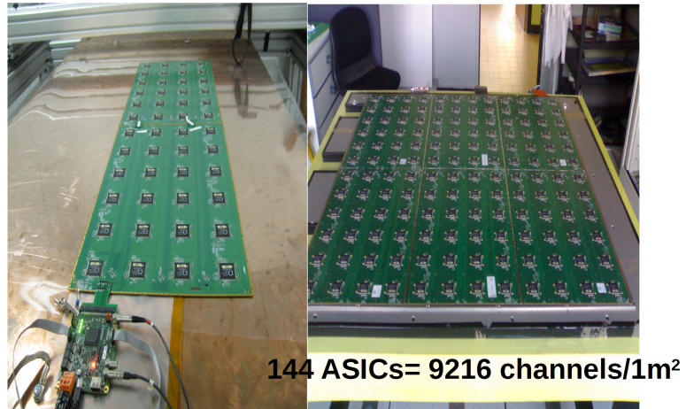
FIGURE 3.6: The electronic of 1m 2 GRPC composed by 6 ASUs (left) and one slab of two ASUs connected to the DIF (right).
