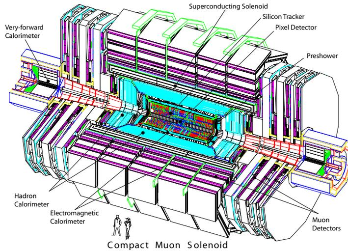
Figure 2.3: View of the CMS detector. Main elements are labelled.
