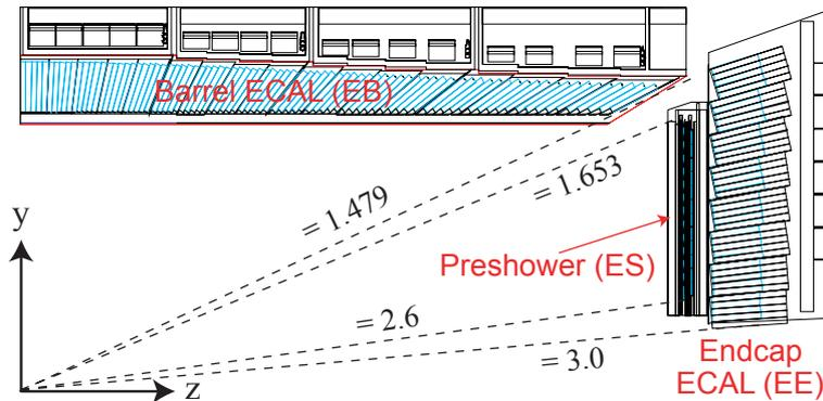
Figure 2.5: The electromagnetic calorimeter and the preshower.
