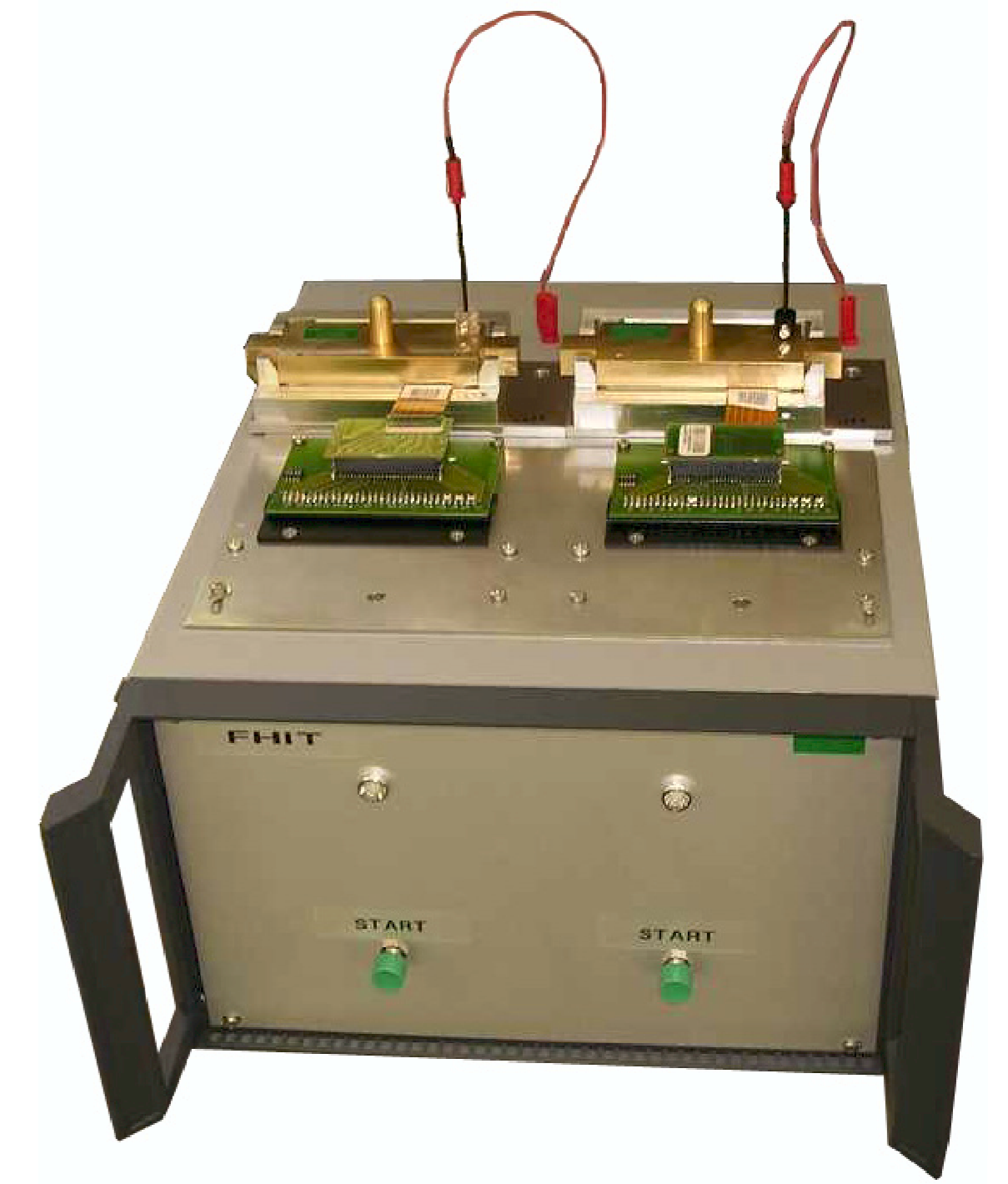
Figure 5: Front-end Hybrid Industrial Tester (FHIT) setup with 2 hybrids during a dual test in industry.
